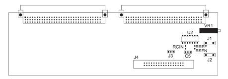
VR1 is used to adjust the LCD voltage, VLCD.
