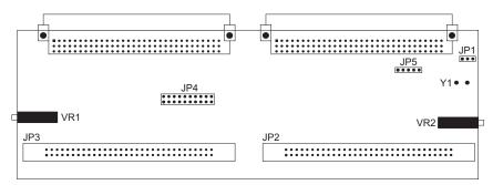
The external clock source has two modes, RC and Crystal. If a crystal clock is to be used, positions 2 and 3 should be shorted on JP1 and a suitable crystal inserted into location Y1. Otherwise, if an RC clock is to be used, positions 1 and 2 should be shorted and the system frequency adjusted using VR2. Refer to the Tools/Mask Option menu of the HT-IDE3000 User's Guide for the clock source and system frequency selection. VR1 is used to adjust the LCD voltage, VLCD.
