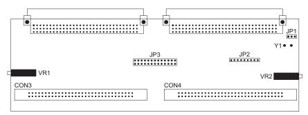
The external clock source has two modes, RC and Crystal. If a crystal clock is to be used, positions 2 and 3 should be shorted on JP1 and a suitable crystal inserted in location Y1. Otherwise, if an RC clock is to be used, positions 1 and 2 should be shorted and the system frequency adjusted using VR2. Refer to the Tools/Mask Option menu of the HT-IDE3000 User's Guide for the clock source and system frequency selection. VR1 is used to adjust the LCD voltage, VLCD.
