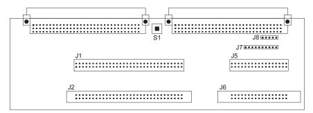
Switch S1 is used to simulate a low voltage condition, a situation which can be detected internally by the HT95L400/40P, HT95L300/30P, HT95L200/20P and HT95L100/10P devices. When switch S1 is pressed, the low battery flag (LBFG; bit 4 of LCDC register) will be set, resulting in a simulated low battery condition.
