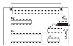
The external clock source has two modes, RC and Crystal. If a crystal clock is to be used, positions 2 and 3 should be shorted on JP1 and a suitable crystal inserted into location Y1. Otherwise, if an RC clock is to be used, positions 1 and 2 should be shorted and the system frequency adjusted using VR1. Refer to the Tools/Mask Option menu of the HT-IDE3000 User's Guide for the clock source and system frequency selection.
