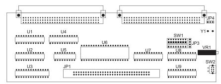
The external clock source has two modes, RC and Crystal. If a crystal clock is to be used, positions 2 and 3 should be shorted on JP4 and a suitable crystal inserted into location Y1. Otherwise, if an RC clock is to be used, positions 1 and 2 should be shorted and the system frequency adjusted using VR1. Refer to the Tools/Mask Option menu of the HT-IDE3000 User's Guide for the clock source and system frequency selection.
