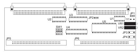
The external clock source has two modes, RC and Crystal. If a crystal clock is to be used, positions 2 and 3 should be shorted on JP1 and a suitable crystal inserted into location Y1. Otherwise, if an RC clock is to be used, positions 1 and 2 should be shorted and the system frequency adjusted using VR1. Refer to the Tools/Mask Option menu of the HT-IDE3000 User's Guide for the clock source and system frequency selection. VR2 is used to adjust the LCD voltage, VLCD.
