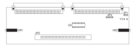
The external clock source has two modes, RC and Crystal. If a crystal clock is to be used, positions 2 and 3 should be shorted on JP1 and a suitable crystal inserted into location Y1. Otherwise, if an RC clock is used, positions 1 and 2 should be shorted and the system frequency adjusted using VR2. Refer to the Tools/Mask Option menu of the HT-IDE3000 User's Guide for the clock source and system frequency selection. VR1 is used to adjust the LCD voltage, VLCD.
