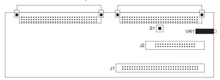
VR1 is used to adjust the LCD voltage, VLCD.
