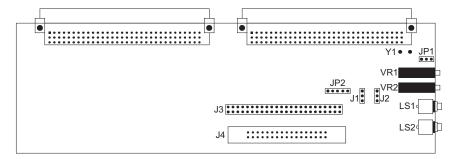
The external clock source has two modes, RC and Crystal. If a crystal clock is to be used, positions 2 and 3 should be shorted on JP1 and a suitable crystal inserted into location Y1. Otherwise, if an RC clock is to be used, positions 1 and 2 should be shorted and the system frequency adjusted using VR1. Refer to the Tools/Mask Option menu of the HT-IDE3000 User's Guide for the clock source and system frequency selection.
